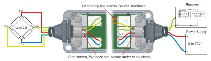
The input and output cable screens should be dressed back onto each cable respectively with 360° coverage then the cable clamps fitted to provide both screen continuity through the PCB and cable strain relief.
