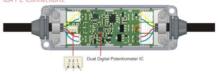
To connect to the I<sup>2</sup>C programming connector on the ILA, an ILA-CAB-A cable assembly is available from Mantracourt.
