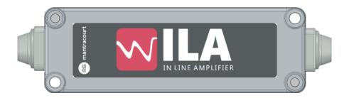
Housed in an IP54 in-line enclosure, Mantracourt's In-Line Amplifier (ILA) converts strain gauge or load cell inputs into a high stability 4-20 mA output. Its small design enables it to be easily integrated into compact installations. The ILA is compatible with a wide range of inputs including strain gauges, load cells, pressure and torque transducers.
