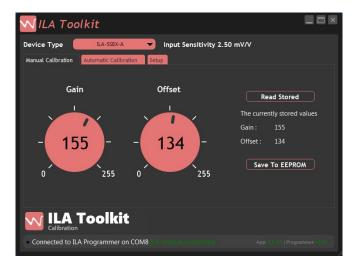
The Gain and span controls indicate the current settings of the two potentiometers within the extreme values of 0 to 255.
