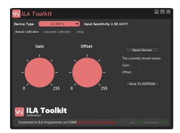
With the connections all in place, the virtual potentiometers can be 'rotated' throughout their range by first clicking on them then grab-and-dragging their pointers with the mouse or clicking and using the mouse wheel to increment or decrement their positions. The latter method allows finer control.
