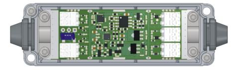
The grommets cater for cable diameters between 4 to 6 mm. Smaller diameter cables can be used at the expense of effective dust and particle sealing.
