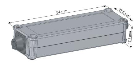
The grommets increase the overall length to 94 mm
