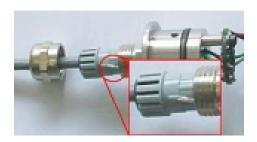
8. Taking care not to damage the EMC 'O' ring, and making sure that the cable drain wire passes back through the gland, carefully assemble the enclosure body with the PCB mounted on it, to the enclosure cover and fit the two retaining grub-screws.
