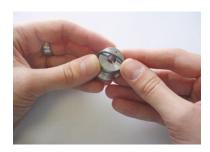
3. Lay the cable drain wire back along the cable outer insulation and pass the prepared end of the cable through the gland shell on the enclosure body.
