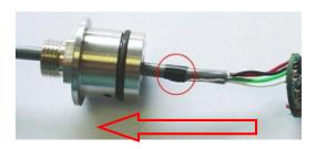
7. Push the plastic insert fully home and check to ensure that no strands from the drain wire are visible; slide the gland nut into place and tighten so that the cable is firmly gripped by the lining of the plastic insert.
