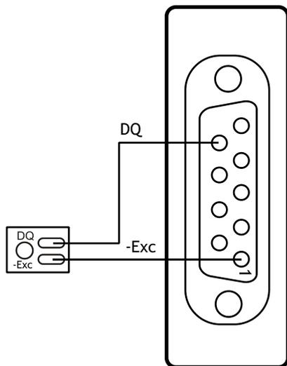
The temperature module is a small double sided PCB with an 8 pin SOIC integrated circuit mounted to it. The dimensions are 10.5 x 7.6 x 2.5mm (0.413 x 0.299 x 0.098"). There are two solder pads for connection to the DSCUSB-PT. A 2mm hole is used for fixing the temperature module to the body of the load cell.
