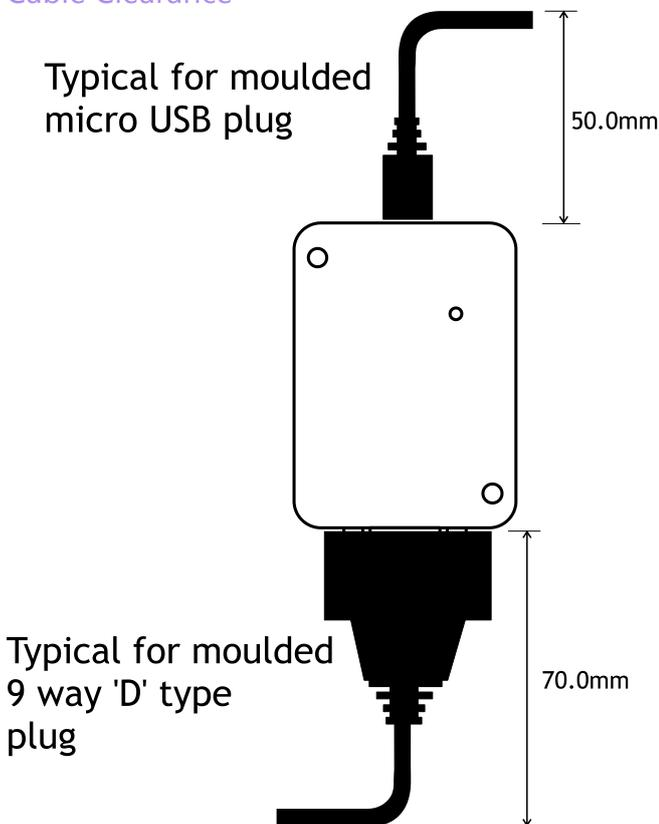
These are typical clearances but smaller mouldings or using a tighter cable radius can reduce this.
