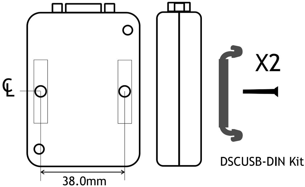
A DIN rail mounting kit is available for top hat DIN rail EN 50022. Optional part DSCUSB-DIN consists of a pair of screws and two DIN rail clips.
