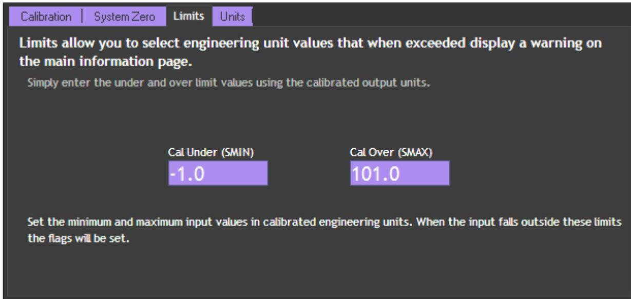
The screenshot shows a software interface with a dark background and light text. At the top, there is a navigation bar with four tabs: 'Calibration', 'System Zero', 'Limits', and 'Units'. The 'Limits' tab is currently selected. Below the navigation bar, the main content area contains the following text:
