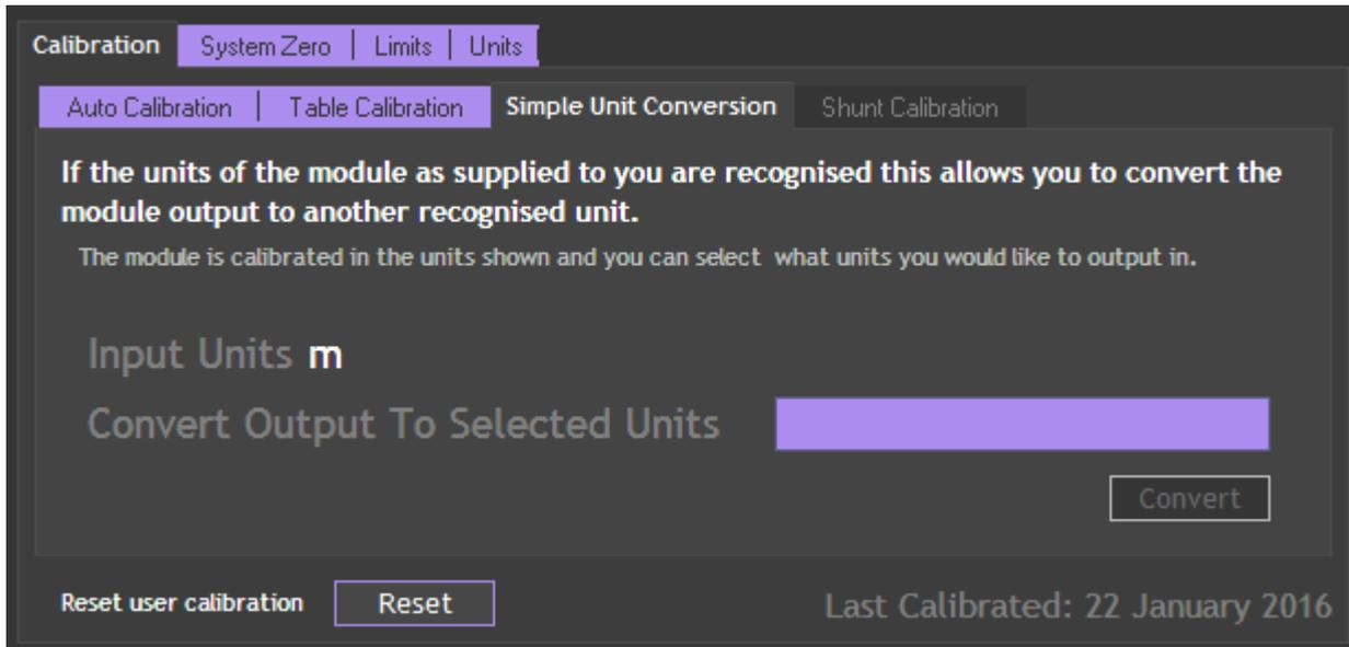
This tab will only be enabled if the module has been calibrated in the Advanced Calibration section.
