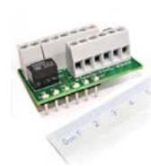
SGABCM Bridge completion module for both quarter and half bridges, compatible with all versions of SGA
