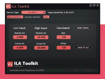
With auto calibration, you set the mA required against the actual mA. The gain and offset values are calculated based on input required.
