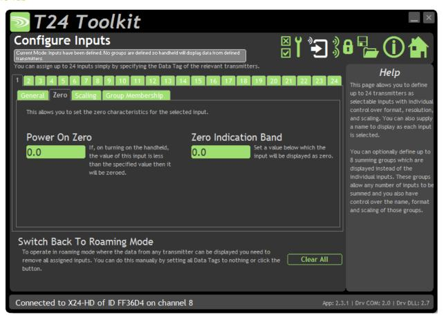
Here you can configure the zero settings for the selected Transmitter input.
