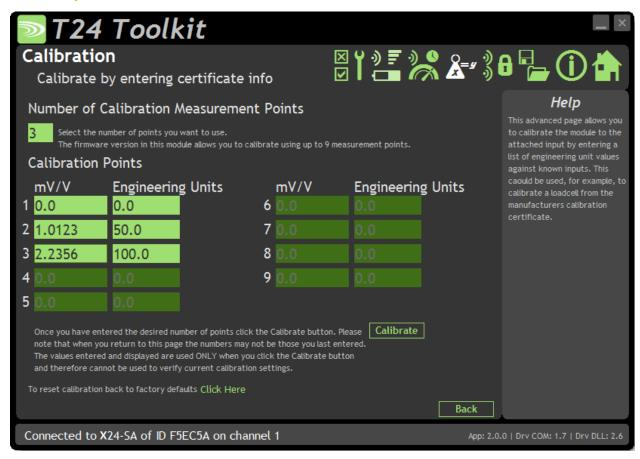
In some circumstances it may not be possible to apply inputs in which case the calibration can be entered manually from the calibration table or certificate for a load cell without ever having to connect the load cell.
