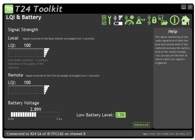
Available for Transmitters only. Here you can see the voltage of the battery and the radio signal levels at the base station and the remote transmitter module. This simple view gives an LQI value which stands for Link Quality Indicator. This value will range from 0 to 100 and within this band you should still achieve communications. As the level drops towards zero communications may become intermittent but still achievable.
