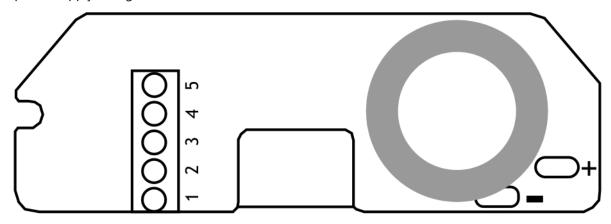
Connect to a 3 V power supply or batteries to the solder pads marked + and -.
