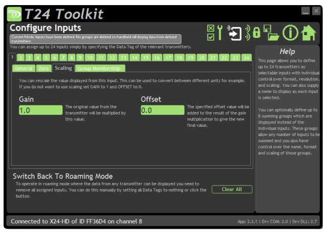
Here you can configure the scaling for the selected Transmitter input.
