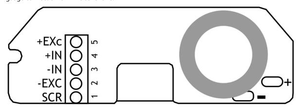
The resistance of the strain gauge can be between 85 and 5000 ohms. The X24-SA can support up to four 350 ohm strain gauges bridges attached in parallel (At the expense of reduced battery life).
