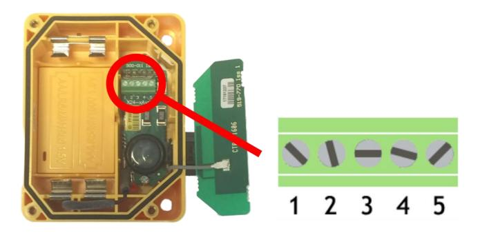
The input connections are accessed by lifting the right hand cover plate, this plate incorporates the X24 Antenna; take extra care when re-assembling that the grey UHF cable is attached to the antenna socket.
