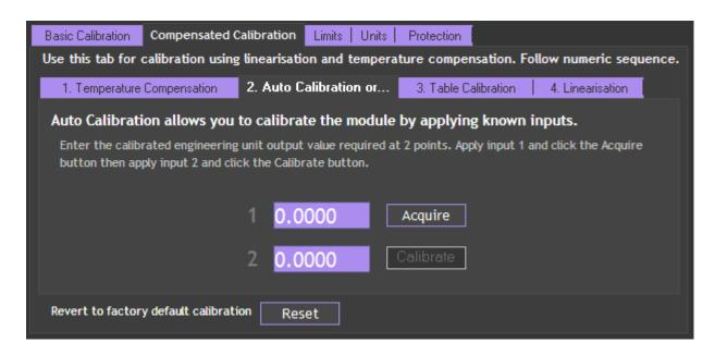
The automatic calibration requires that you apply two known (ascending) inputs in sequence. Just enter the required engineering unit value for the two inputs in the fields marked 1 and 2.
