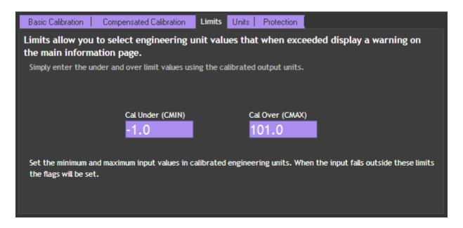
Here you can set limits below and above which the warning indicators will be displayed on the Information Page for the standard user. These limits should cover the operational range that the combined potentiometer and DSCUSB-PT are allowed to operate over.
