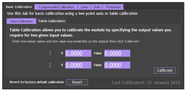
This option lets you calibrate direct from the sensor manufacturers certificate without having to apply inputs to the module.
