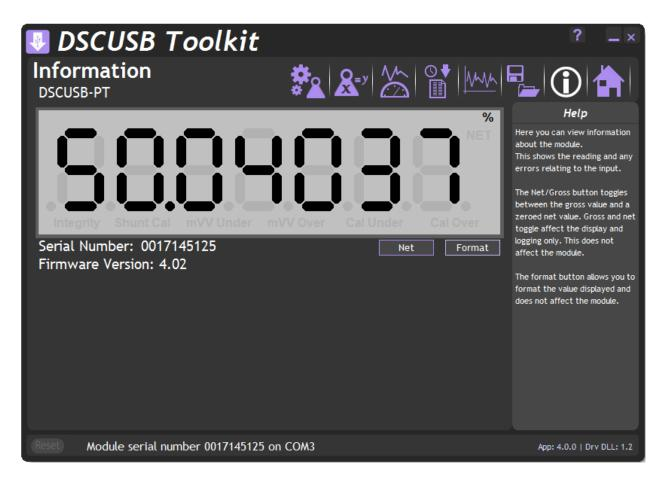
This simply shows a large display and indicates if any error conditions are present by displaying an information box. If the module has been allocated engineering units these may be displayed in the upper right of the LCD display.
