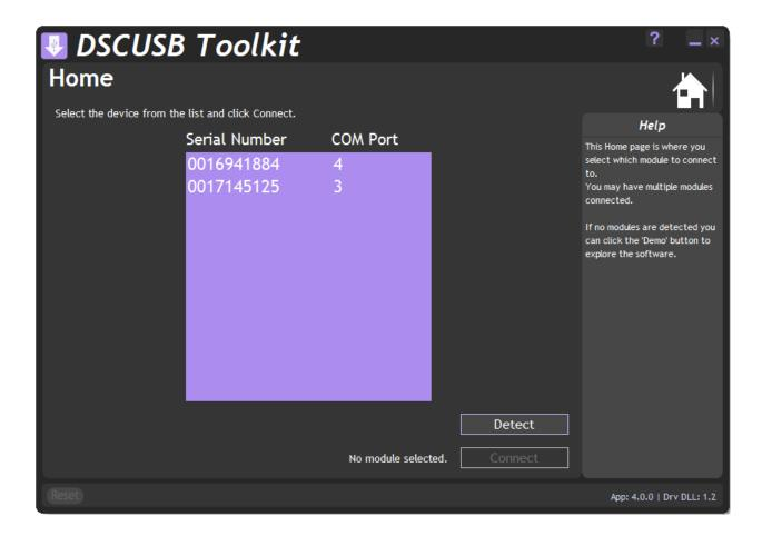
You can then select a different module or plug in a different module. If you change the connected modules click the '**Detect'** button to re-list the modules. Then select the required module from the list.
