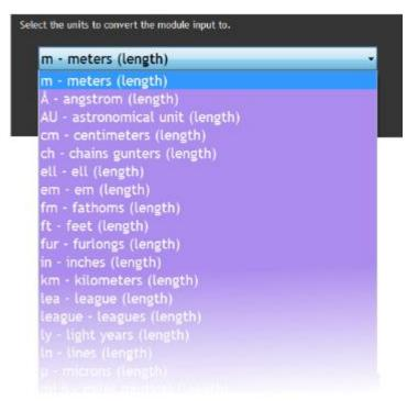
Select the required units, click OK then click the 'Convert' button. The Toolkit will then alter the user calibration to provide the output in the selected engineering units.
