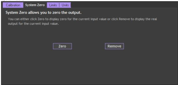
To remove the current value on all subsequent readings click the '**Zero'** button. Click the '**Remove'** button to return to displaying the actual input applied. This system zero is stored in the module and remains through power cycling.
