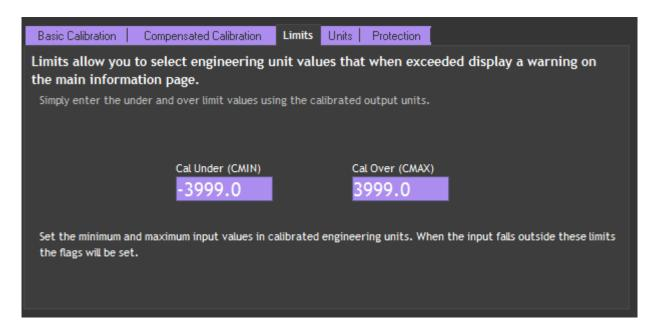
Here you can set limits below and above which the warning indicators will be displayed on the Information Page for the standard user. These limits should cover the operational range that the combined loadcell and DSCUSB are allowed to operate over.
