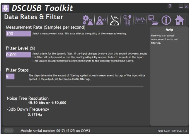
Here you can configure how fast the module generates new results. The faster the new results are generated the lower the effective noise free resolution will become. The software will show you the expected noise free resolution achievable with your settings.
