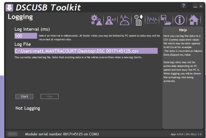
Log data to a CSV file at intervals of between 10 milliseconds and 32 seconds. This allows data to be logged at up to 100Hz and the resulting CSV files can then be analysed in Microsoft Excel or similar application.
