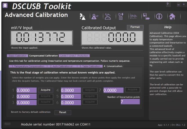
Linearised calibration in your chosen engineering units can be achieved by applying known inputs or entering values from a sensor calibration certificate. You can also calibrate the Shunt Calibration so an installed system will always give an output of 100 when Shunt Calibration is activated. This allows for an extremely fast check that your system is still operating correctly without having to disconnect the input sensor.
