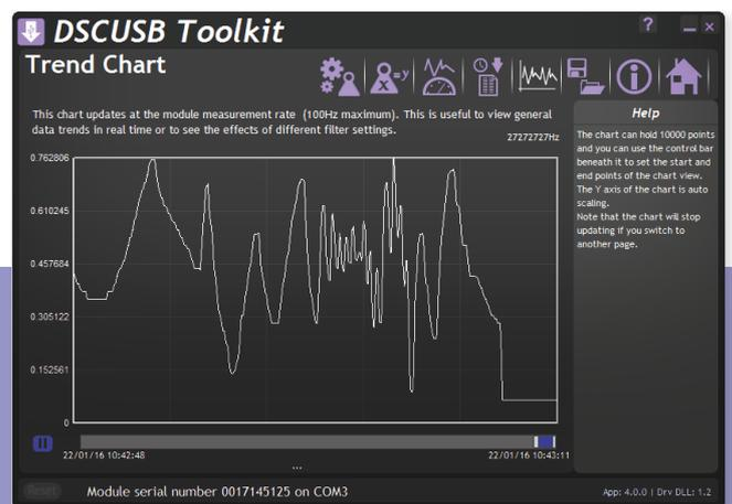
Feature a real-time scrolling graphic display. The chart can hold up to 10,000 points and you can zoom and pan through the data. The chart is auto scaling and is ideal for looking at input signals to allow tuning the filters.
