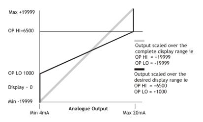
Method of Calculating Output Low & Output High from known output values
