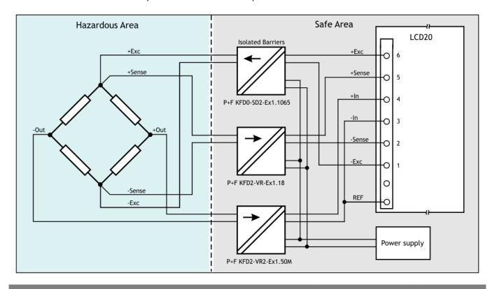
D Because the barriers are fully isolated, the **REF** connection <u>MUST</u> be made to ensure that the LCD20 input stage is biased correctly.
