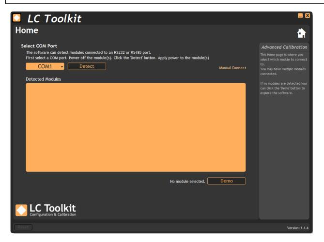
The serial ports (COM ports) on the computer are detected and added to the drop down list on the top left of the page. Clicking the drop down list will automatically re-detect available COM ports. To detect the connected module:
